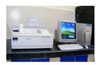
The Lambda 25 UV-visible spectrometer is provided with double beam optics, which incorporates concave holographic grating along with a proven optical design to minimize stray radiation with accurate results. The system has a noise specification of 0.0003A peak to peak, which means that 0.0003A is the lowest usable absorbance reading. The optical performance of the lambda series ensures that you will get dependable results at high and low absorbance
