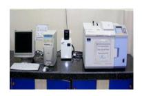
Gas chromatography is a technique used for separation of volatile substances, or substances that can be made volatile, from one another in a gaseous mixture at high temperatures. This method depends upon the solubility and boiling points of organic liquids in order to separate them from a mixture. It is both a qualitative (identity) and quantitative (how much of each) tool.
